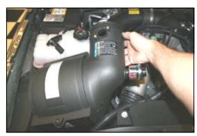
**4.** Slide the flexible intake tube off of the factory airbox and then rock the airbox back and forth to free it from the mounting grommets, next lift it straight up and remove it from the vehicle.
