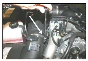
1. <u>Disconnect the negative battery cable.</u>
