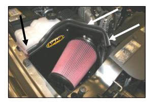
**13.** Install the Airaid Premium Filter (#1) onto the Airaid intake tube (#4), and tighten the hose clamp. Now install the provided weather strip (#5) on the top of the **CAD**. Apply the Airaid Foil Decal onto the Panel as shown.
