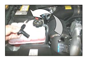
**3.** Without disconnecting the wiring harness, remove the Mass Air Flow sensor from the factory airbox, and set it aside.
