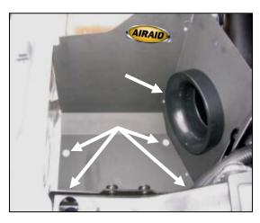
7. Install the air filter adapter (#4) using three ½-20x ½" button head bolts (#12), and 1/4" flat washers (#13). Position the Airaid Cool Air Dam in place of the factory airbox & secure it with four M6-1x25 hex bolts (#14) and 1/4" flat washers (#13). Apply the Airaid Decal as shown.
