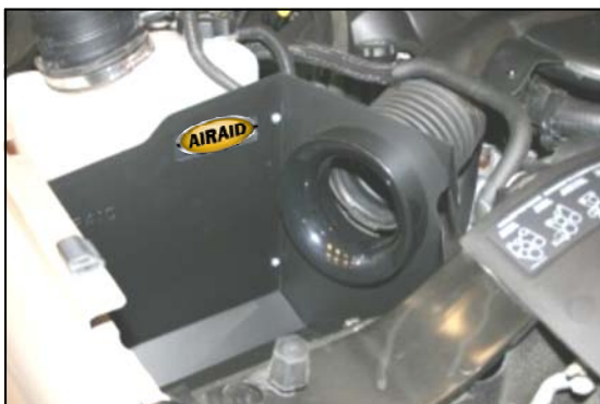
8. Install the assembled CAD in place of the factory airbox using four bolts (#8) and washers (#7). Do not over tighten the bolts.
