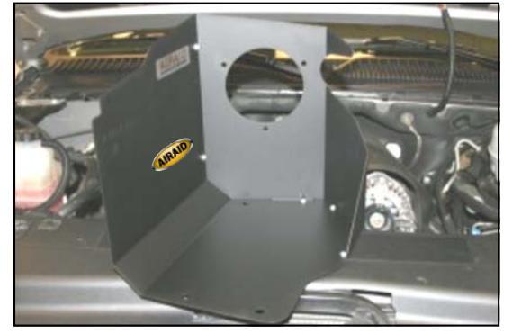
6. Assemble the two Cool Air Dam panels (#2) and (#3) using the five supplied screws (#9), washers (#10), and nuts (#11), as shown.
