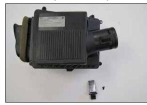
15. Remove the mass air sensor from the factory air box.
