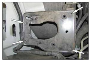
7. Remove the four bolts securing the air box mounting tray and then remove the tray from the vehicle. **NOTE: Three of the bolts will be reused in a latter step.**
