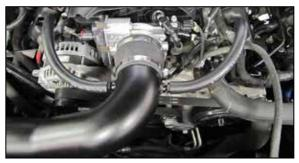
19. Connect the provided crank case vent hoses to the ports on the valve covers and then connect the open ends to the fittings installed into the AIRAID intake tube.
