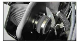
14. Install the coupling hose (08699) to the filter adapter and secure with the provided hose clamp.
