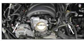
12. Remove the two factory crank case vent tubes from the vehicle.
