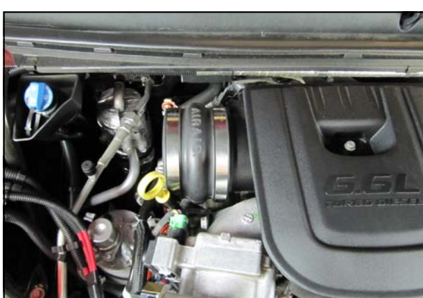
8. Slide the Hump Hose and Clamps onto the turbo inlet. Leave the clamps loose for now.
