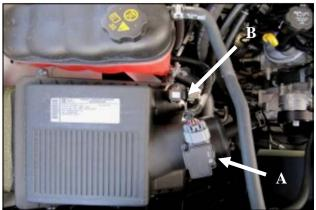
5. Disconnect the Mass Air Flow or MAF sensor (  $\bf A$  ) and the Manifold Absolute Pressure or MAP sensor (  $\bf B$  ) Remove the factory airbox from the vehicle.
