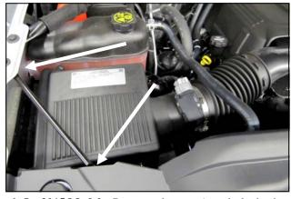
**6.** On 2015 Models: Remove the two 6mm bolts in the fender brace and set the bolts and brace to the side.
