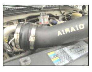
**11.** Install the urethane hump hose (#5) and two #72 hose clamps (#12) onto the large end of the Airaid Intake tube. (*Note: Leave hose clamps loose until final assembly.*)
