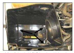
**6.** Install the Airaid **CAB** into the vehicle replacing the factory airbox. Secure the **CAB** using Three of the factory bolts from step 4. Do not over tighten Apply the Airaid Bubble Decal inside the Airbox as shown.
