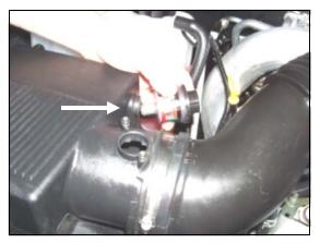
2. Remove the factory filter minder and grommet from the side of the factory airbox (save for re-
