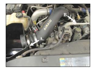
**13. A.**) Install the hump hose end of the Airaid intake tube assembly onto the filter adapter first. **B.**) Slip the coupler end of the tube over the factory turbocharger inlet. Adjust for fit, and tighten the hose clamps
