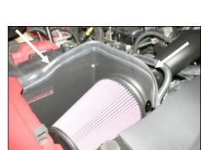
13. Install the Airaid Premium Filter (#1) onto the air filter adapter, and tighten the hose clamp. Next install the provided weather strip (#9) onto the top of the CAD. For ease of install, start at the inner fender, and work your way towards the radiator. Reinstall the beauty cover.
