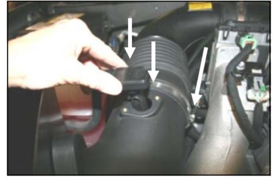
**12.** Re-position the factory intake tube onto the Airaid tube, and tighten the hose clamp. Next re-install the Mass Air Flow sensor into the Airaid tube **using the two provided Button Head screws (#8).** Do not use the factory screws! Do not over tighten!
