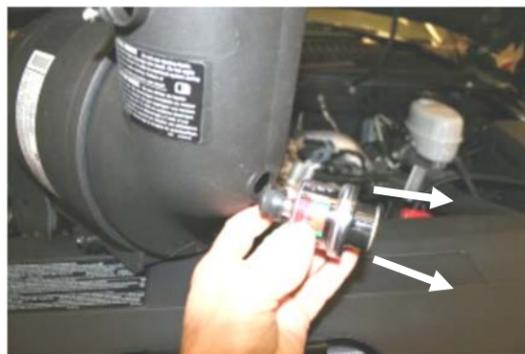
**5.** Remove the factory filter minder and grommet from the factory airbox. Save them for later use.
