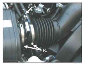
1. Disconnect the negative battery cable. A.) Disconnect the Mass Air Flow (MAF) sensor wiring harness.
