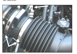
7. Slide the MAF sensor onto the filter adapter and tighten the clamp. Slide the factory intake tube onto the other side of the MAF sensor, and tighten the clamp. Reconnect the MAF sensor wiring harness.
