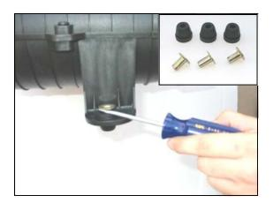
**3.** Remove the factory airbox and set it aside. Using a flat blade screwdriver, remove and save the three factory rubber grommets and inserts from the airbox base.
