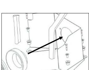
**5.** Install the filter adapter (#4) into the Airaid Cool Air Dam using three 1/4-20x 5/8" bolts (#6), and 1/4"
