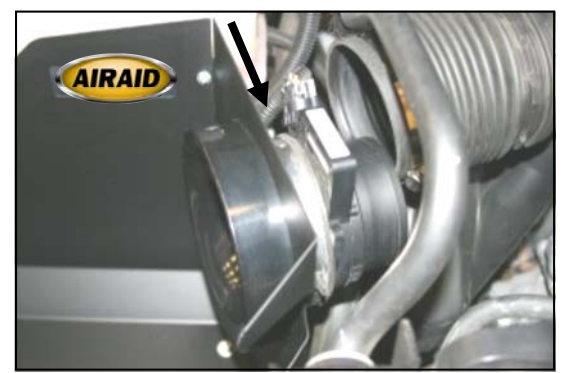
9. Re-install the Mass Air Sensor and coupler onto the air filter adapter (#4), as shown and tighten the hose clamp.
