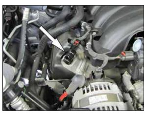
10. Install the provided 90° quick disconnect fitting onto the valve cover PCV port.
