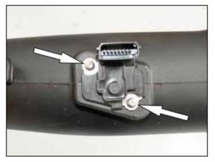
7. Remove the OEM mass air sensor from the factory air filter housing and install it into the AIRAID<sup>®</sup> intake tube and secure with the provided hardware.
