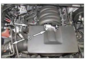
1. **Disconnect the negative battery cable!** A. Depress the grey locking tab in the PCV breather connector quick disconnect fitting on the valve cover and disconnect the PVC from the valve cover. B. Loosen the hose clamps that secure the intake plenum assembly to the throttle body and air filter housing and then remove the complete assembly from the vehicle.
