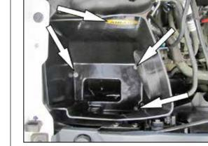
5. <u>Install the AIRAID air box into the vehicle</u> and secure with three of the OEM bolts from step #3. Apply one of the provided AIRAID<sup>®</sup> decals to the air box as shown.
