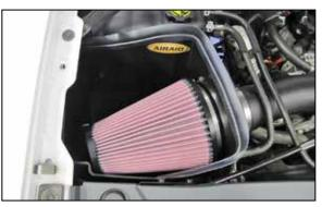
14. Install the weather strip onto the top edge of the AIRAID<sup>®</sup> air box with the contour rolling away from the filter as shown.
