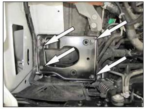
3. Remove the four bolts shown securing the air filter housing tray to the inner fender and then remove the tray from the vehicle. **NOTE: Three of these bolts will be reused in a later step.**
