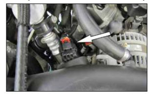
12. Reconnect the mass air sensor and secure the red locking tab.
