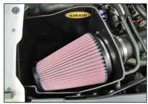
13. Install the AIRAID® air filter onto the filter adapter and secure with the provided hose clamp.
