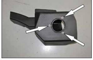
4. <u>Install the filter adapter</u> into the AIRAID<sup>®</sup> air box and secure with the provided hardware.
