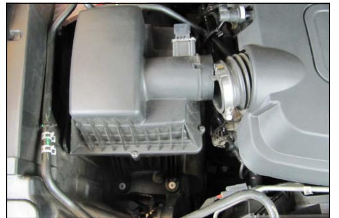
3. Loosen the intake clamp and slide the tube off of the air box lid as shown. Using a screwdriver, remove the air box lid and air filter.
