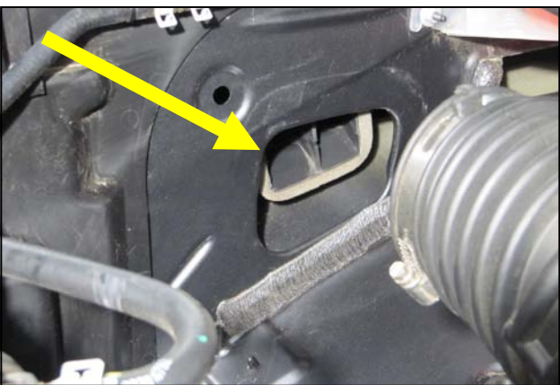
19. On Duramax Powered vehicles, maximum power is achieved by removing the airbox duct in the inner fender.
