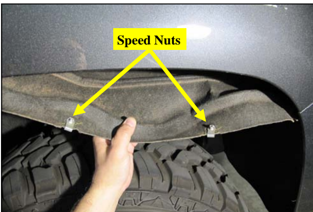
20. Inside the passenger side wheel well, remove the two center screws in the fender liner. Slide back the liner and pull it down. Take caution no to loose the speed nuts.
