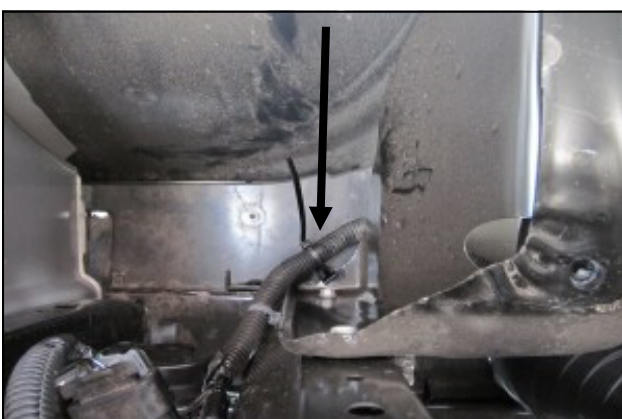
7. Secure the wiring harness to the inner fender as shown using the Edge Clip Cable Tie (#14).
