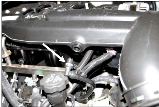
2. Pull the PCV breather line from the factory intake tube.
