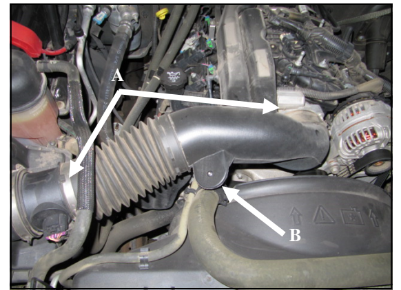
3.A.) Loosen the clamps securing the factory intake tube to the throttlebody and the Mass Air Flow Meter, or MAF. B.) Separate the hose anchor from the factory intake and remove the factory tube.
