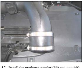
**12.** Install the urethane coupler (#6) and two #60 hose clamps (#11) onto the small end of the Airaid intake tube. (*Note: Leave hose clamps loose until final assembly.*)
