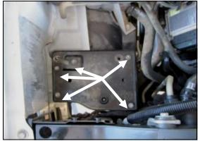
**3.** Using a 10mm socket, remove the five bolts and mounting plate from the engine compartment. Do not discard factory bolts. Three of them will be re used in step 5.
