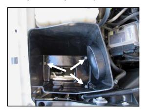
**5.** Install the Airaid Cold Air Box into the vehicle replacing the factory airbox. Secure the CAB using three of the bolts from step 3. Do not over tighten
