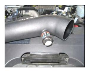
**9.** Transfer the factory rubber grommet and air filter minder from the airbox top into the Airaid intake tube As shown.
