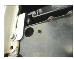
**7.** Install the Fender bracket (#13) as shown. **A.**) Secure the bracket to the fender using the factory bolt. **B.**) Use the 1/4-20 x 3/4" hex bolt (#14), one 1/4" flat washer (#9), and the 1/4-20 flange nut (#15) to secure the **CAB** to the Bracket.
