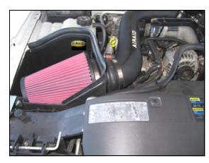
**15.** Install the Airaid Premium Filter (#1) onto the filter adapter, and tighten the hose clamp. Install the weather strip (#7) onto the Airaid Cold Air Box. Reconnect the **M.A.F.** sensor . Apply the Airaid Decal inside of the Airbox as shown.
