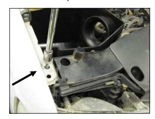
**6.** Using a 13mm socket, remove the factory fender bolt and set it aside. It will be reused in step 7.
