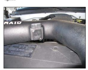
**8.** Transfer the **M.A.F.** Sensor from the factory airbox into the Airaid intake tube (#2). Use the two 8-32 button head screws (#10). to secure the meter.
