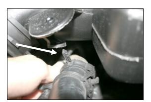
3. Separate the factory intake tube from the plastic clamp that secures the radiator hose to the tube. A firm downward push will usually do it.
