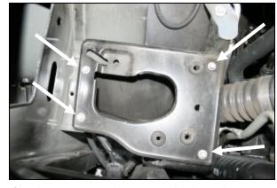
**3.** Using a 10mm socket, remove 4 bolts, and remove the factory air filter mounting plate.
