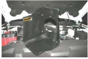
**5.** Assemble the two Cool Air Dam panels (#2) and (#3) as shown, using the five 6-32 screws (#10), washers (#11), and nuts (#12).Apply the Airaid Foil Decal onto the Panel as shown.
