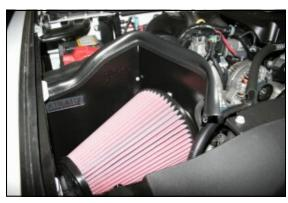
**11.** Install the Airaid Premium Filter (#1) onto the Airaid intake tube (#4), and tighten the hose clamp. Now install the provided weather strip (#5) on the top of the CAD. For ease of installation, start near the fender and work your way towards the radiator.
