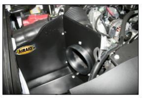
**8.** Install the Cool Air Dam into the vehicle where you removed the factory mounting plate in step #4, using the four supplied M6-1x25 bolts (#9), and flat washers (#7).
