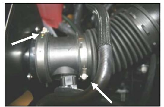
9. Re-install the Mass Air Flow sensor and coupler onto the air filter adapter (#4), as shown and tighten the hose clamp. Next re-connect the factory intake tube to the Mass Air Flow sensor, and tighten the hose clamp.
