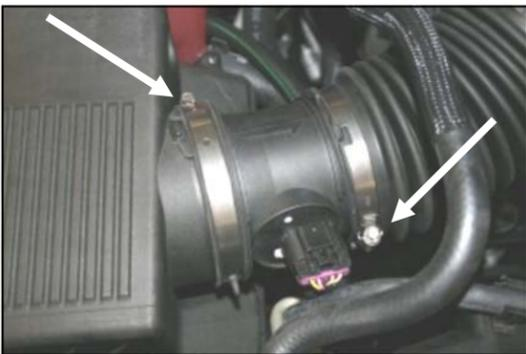
1. **Disconnect the negative battery cable.** Loosen the hose clamp on the end of the factory intake tube at the Mass Air Flow sensor, next loosen the hose clamp that holds the Mass Air Flow sensor to the factory air box.
