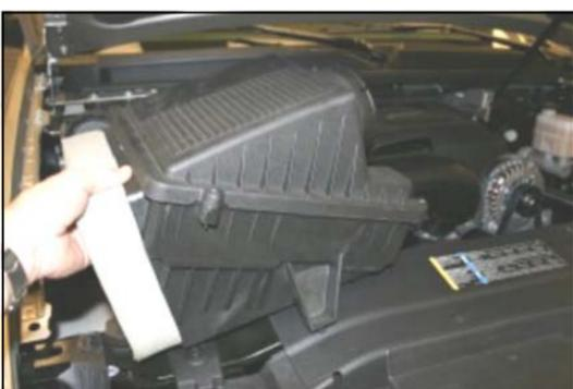
4. Remove the factory air box from the vehicle.
