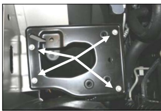
5. Remove 4 bolts, and remove the factory air-box mounting plate.
