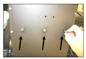
7. Install the three silicone bumpers (#15) into the three holes in the bottom of the Cool Air **D**am, as shown.
