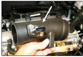
**9.** Install the Mass Air Flow sensor removed in step #4, into the Airaid Intake Tube (#5) using the two 8/32"x 3/8" button head screws (#10).
