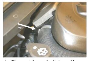
1. **Disconnect the negative battery cable.** With a 1/4" socket, loosen the hose clamp that holds the fresh air intake tube to the factory air cleaner housing. Slip the tube off of the factory air cleaner housing and set it aside, it will be reconnected later in the install.
