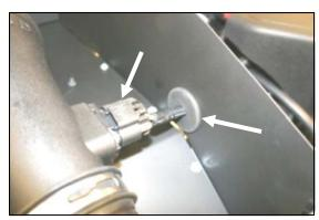
**14.** Re-connect the wiring connector to the **MAF**, and then seat the large grommet into the hole in the side of the **CAD**.
