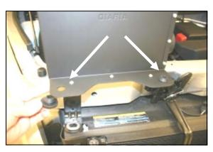
**8.** Install the two large factory grommets removed from the factory air cleaner housing in step #5, into the two holes at the back of the Airaid Cool Air **D**am.
