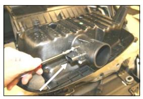
**4.** Using the supplied #20 torx bit, remove two screws, and the **M**ass **A**ir **F**low sensor from the factory air cleaner housing. Set it aside for reinstallation later in the install.
