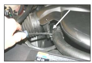
**3.** With a screwdriver, pry the factory tube away from the plastic clamp on the radiator hose, and remove the tube.
