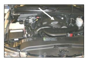
1. **Disconnect negative battery cable.** With a 5/16" socket, remove one bolt on the top of the beauty cover. Set the bolt and the cover aside for re-installation later.
