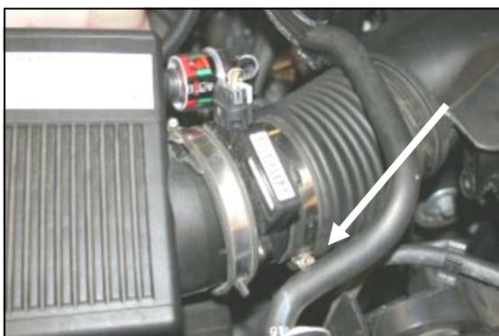
1. Disconnect negative battery cable. Loosen the hose clamp on the end of the factory intake tube at the Mass Air Sensor.
