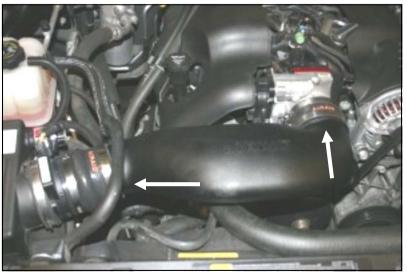
**6.** Install the Modular Intake Tube (#2) into the hump hose first, and then into the throttle body. Adjust for fit, and tighten all four hose clamps. Re-insert the plastic piece from step #3 into the hole on the bottom of the MIT.
