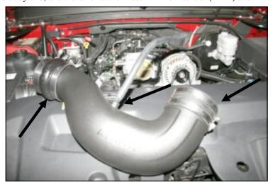
**6.** Install the urethane coupler (#4) on the throttle body end of the Modular Intake Tube (#2) with two #64 hose clamps (#6). Install the urethane hump hose (#3) on the other end of the MIT with the remaining two #64 hose clamps. Leave all clamps loose for now. Install the 3/8" barbed fitting (#7) into the MIT, and slide the 3/8" breather hose (#5) over the barbed fitting as shown.
