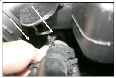
**3.** Separate the factory intake tube from the plastic clamp barb that secures the radiator hose to the tube. A firm downward push will usually do it.
