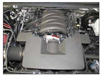
6. Reinstall the factory intake plenum, reconnect the crank case vent lines. **Reconnect the negative battery cable!**
