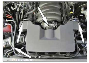
1. **Disconnect the negative battery cable!** Disconnect the crank case vent line quick disconnect fittings from the intake plenum. Loosen the two hose clamps that secure the intake plenum to the throttle body and to the air filter housing, then remove the intake plenum from the vehicle.
