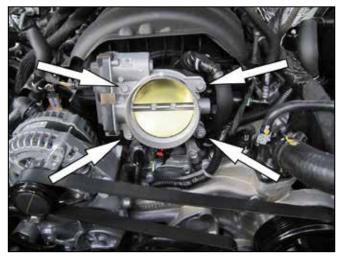
4. Remove the four bolts that secure the throttle body to the intake manifold. Pull the throttle body away from the intake manifold without disconnecting the wiring harness.
