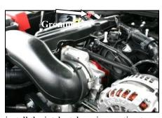
9. Re-install the intake tube using caution to center the intake tube hole over the previously installed grommet. Some adjustment may be required to seat the grommet correctly back into the intake tube. Tighten the hose clamps on the tube. Re-connect the breather tube. Re-install the plastic holder from step #1. Re-install the beauty cover. Re-connect the negative battery cable!
