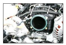
**4.** Using a 4mm socket, remove the two studs that held the throttle body to the intake manifold.
