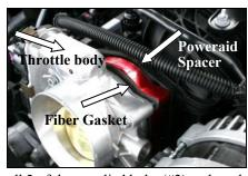
5. Install 2 of the supplied bolts (#2) and washers (#3) thru the two holes in the top of the throttle body, thru the supplied fiber gasket (#4), thru the Poweraid Spacer, and into the two brass inserts in the intake manifold. Run the bolts in a few threads with your fingers. Use caution not to cross-thread the bolts. Next install the 2 remaining bolts (#2) and washers (#3) in the two bottom holes of the throttle body, and tighten in a cross pattern to the vehicle manufacturer's specifications.
