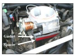
5. Place the fiber gasket (#9) between the Poweraid spacer (#1) and the throttle body. Make sure the flat face of the Poweraid spacer is against the throttle body with the bore extending into the intake manifold. Use caution to retain the factory o-ring gasket on the intake manifold.
