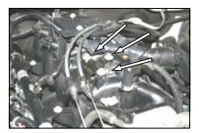
4. If you have an electronic throttlebody, (no cables) skip to step #6. Using a 5/16" socket, remove and save 3 bolts that hold the throttle cable bracket to the intake manifold. (Disregard steps #4, #5, and #8, if you are working on a 8.1L).
