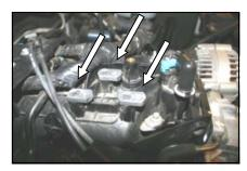
**5.** Install three 1/2" extension plates (#5) using the provided flat head countersunk bolts(#6). Point the long end towards the radiator, and snug them down.
