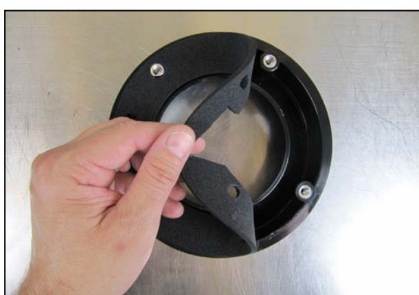
5. Prepare the Filter Adapter for installation by mating the Gasket to it. Note: The Filter Adapter and related parts have an asymmetrical bolt hole pattern.
