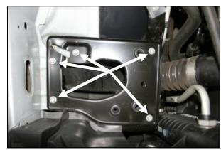
**3.** Using a 10mm socket, remove 5 bolts, and then remove the factory air filter mounting plate.
