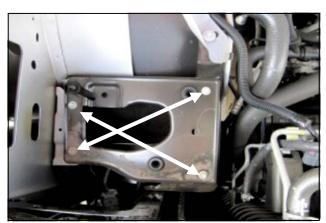
**7.** Remove the four tray bolts and the airbox mounting tray. Three of the bolts will be reused in step **9.**
