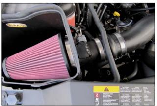
14. Install the Airaid Premium filter (#1) onto the Filter Adapter, and tighten the hose clamp. Reconnect the MAF And MAP sensors. Install the Weather Strip (#8) onto the Airaid Cold Air Box. (<u>Hint</u>: Start from one corner and work your way around for ease of install.)
