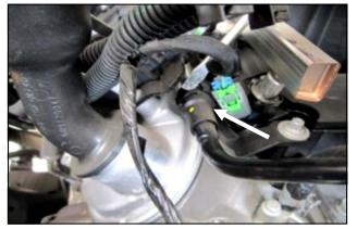
**4.** Remove the plastic PCV breather line from the factory hard line. A standard screwdriver works well for depressing the locking tab in the coupling.
