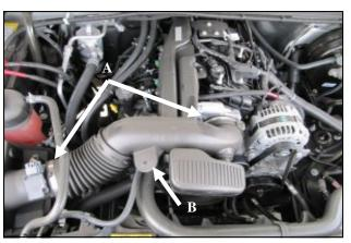
**3.A.)** Loosen the clamps securing the factory intake tube to the throttlebody and the airbox.
