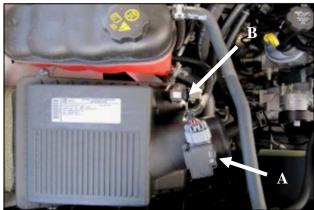
5. Disconnect the Mass Air Flow or MAF sensor ( A ) and the Manifold Absolute Pressure or MAP sensor ( B ) Remove the factory airbox from the vehicle.
