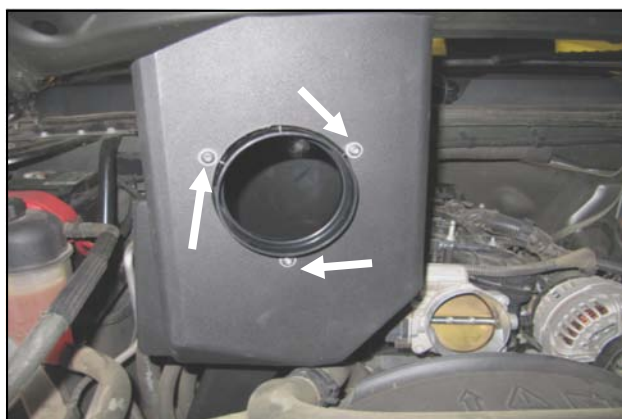
8. Install the Filter Adapter (#4) onto the Cold Air Box or CAB (#3) as shown using the three 1/4-20 Button Head Screws (#9) and 1/4" Flat Washers (#10).
