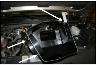
**6.** Install the filter adapter (#4) into the Cool Air Box (#3) as shown using three 1/4" Button head bolts (#8) and three 1/4" flat washers (#11). Next, fasten the bracket (#15) to the front of the **CAB** as shown using one 1/4-20 hex bolt (#9) two flat washers (#10), and one 1/4" Nylock nut. Refer to the drawing above for reference.
