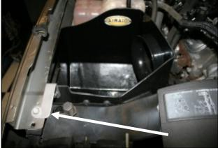
**8.** Install the **CAB** assembly into the vehicle where the factory airbox used to be using three 6mm hex bolts (#12) and three flat washers (#11) thru the bottom. Now reinstall the factory fender bolt thru the bracket and into the fender. Adjust the assembly for fit and tighten all bolts and nuts at this time. Apply the Airaid Foil Decal onto the Panel as shown.
