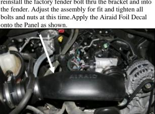
11. Install the small end of the intake tube into the hump hose first and then rotate it slightly to slide the other end into coupler on the throttlebody. Adjust for fit, and then tighten all four hose clamps.
