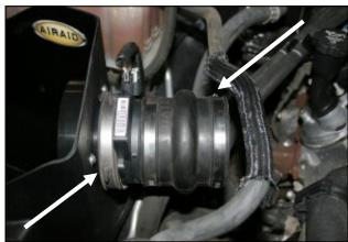
**9.** Reinstall the **MAF** sensor and coupler onto the filter adapter and tighten the clamp.
