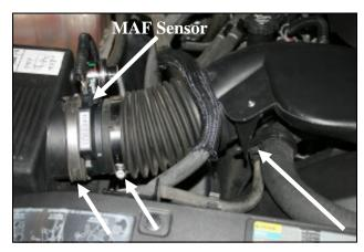
2. Loosen two hose clamps. One on each side of the Mass Air Flow (MAF) sensor.
