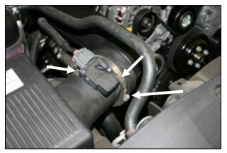
1. Disconnect the negative battery cable. Using a T15 Torx bit, remove the two screws that hold the Mass Air Flow (MAF) sensor to the airbox lid. Next, loosen the hose clamp that secures the intake tube to the lid.
