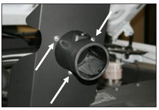
6. Install the filter adapter into panel #3 as shown, using three 1/4-20 x 1/2" button head bolts (#10), and three flat washers (#11).
