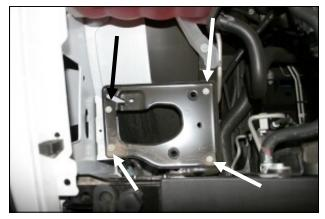
4. Using a 10mm socket, remove the four bolts that secure the factory airbox mounting plate. Now remove the mounting plate from the vehicle.
