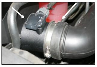
**8.** Reinstall the **MAF** sensor onto the filter adapter using two 8-32 x 5/8" button head screws (#9). **Do Not Use The Factory Screws!** Reconnect the factory air intake tube to the filter adapter and tighten the hose clamp.
