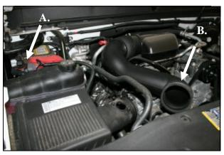
2. A.) Without disconnecting the wiring harness, remove the MAF sensor from the airbox lid and swing it back out of the work area. B.) Now disconnect the factory air intake tube from the airbox lid, and move it out of the work area. V-8 Models: Remove the factory intake tube for ease of install.
