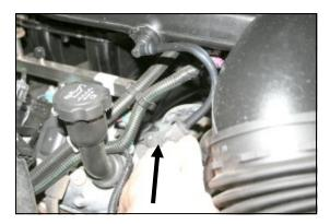
**2.** Disconnect the factory breather hose at the valve cover by pulling the small black tab on the fitting towards the front of the vehicle, and then to the right.
