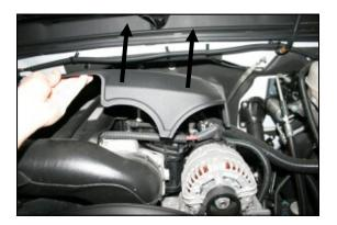
**1. Disconnect the negative battery cable.**Remove the factory beauty cover by lifting up on the front, and then pulling the cover towards the front of the vehicle. It is only held in place by grommets.
