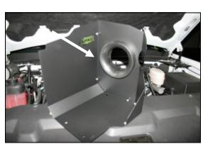
**8.** Assemble the Cool Air Dam panels (CAD) (#2 & #3) using five 6-32 x 5/16" screws (#10), #6 flat washers (#11), and 6-32 keps nuts (#12). Next install the air filter adapter (#5) into the panels as shown with the hole for the Mass Air Flow sensor facing up, using three 1/4 - 20 x 1/2" button head bolts (#14), and 1/4" flat washers (#15). Apply the Airaid Foil Decal onto the Panel as
