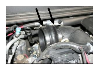
**5.** Install two #72 hose clamps (#10) onto the urethane hump hose (#4), and then slip the hump hose onto the end of the factory turbo intake tube as shown. Leave the clamps loose for now.
