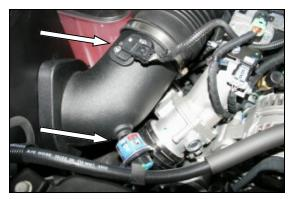
**10.** Reinstall the Mass Air Flow Sensor into the Airaid Intake Tube using the supplied 8-32x1/2" button head screws (#8).
