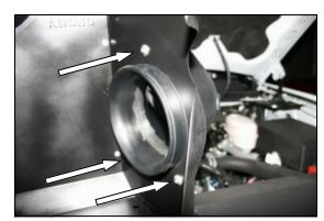
**6.** Install the Airaid intake tube (#4) into the Cool Air Dam using the three 1/4"-20x1/2" button head bolts (#6), and washers (#7) as shown.
