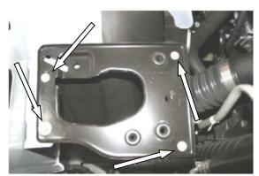
**4.** Using a 10mm socket, remove 4 bolts from the factory airbox mounting plate. Remove the plate from the vehicle.
