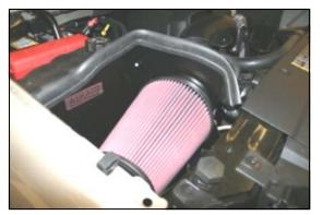
**10.** <u>Install the Airaid Premium Filter</u> (#1) onto the filter adapter (#4), and tighten the hose clamp. Next install the weather strip (#5) onto the top of the **CAD** as shown. For ease of installation start at the fender, and work towards the radiator.
