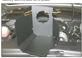
**7.** Assemble the two Cool Air **D**am panels (#2) and (#3) using the five supplied screws (#12), washers (#13), and nuts (#14), as shown.
