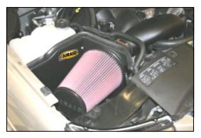
13. Install the Airaid Premium Filter (#1) onto the filter adapter (#5), and tighten the hose clamp. Next install the weather strip (#8) onto the top of the CAD as shown. For ease of installation start at the fender, and work towards the radiator.
