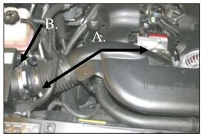
**2.** A.) Loosen the hose clamps on both ends of the factory intake tube. B.) Next loosen the hose clamp on the Mass Air Flow sensor where it clamps on the factory airbox.
