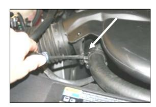
**3.** With a screwdriver, pry the factory tube away from the plastic clamp on the radiator hose, and remove the tube.
