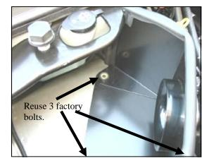
**6.** Install the Airaid Cool Air Dam over the three factory mounting points, and fasten with the factory bolts saved in step #2.
