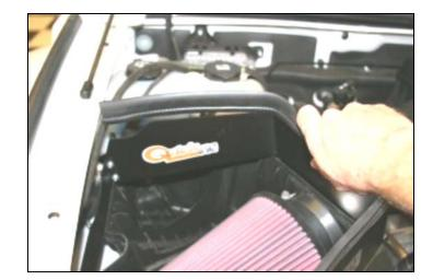
**8.** Starting at one end of the Quick Fit Panel, install the weather strip (#4) as shown.
