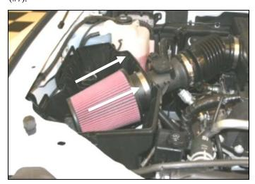
**6.** Make sure the filter and the hose clamp are pushed close to the factory airbox wall, and tighten the hose clamp as shown. **Do Not over tighten.**
