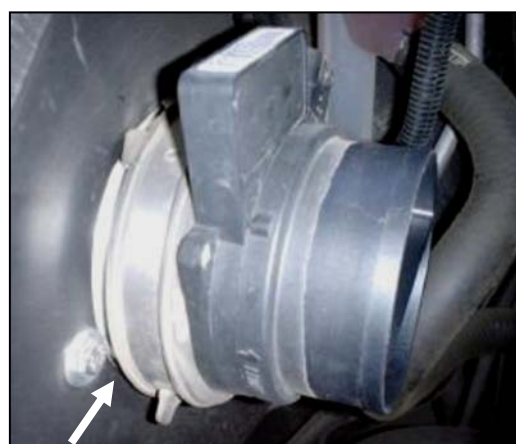
8. Slide the factory MAF sensor onto the air filter adapter and tighten the hose clamp. (Note: factory clamp / rubber bushing must be in place on the inlet to the MAF sensor.)
