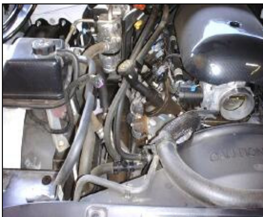
4. Rock the factory air box back and forth and remove it from the vehicle. There are only grommets holding it in, no bolts.
