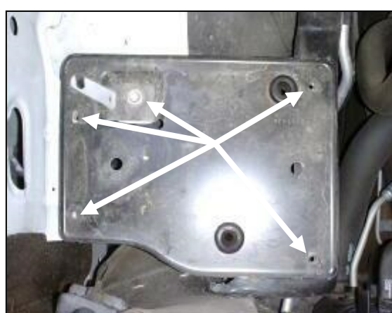
5. Using a 10mm socket, remove the five bolts that secure the factory air filter housing platform and remove it.
