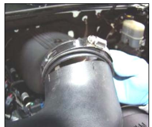
9. Install the GM coupler (#7) onto the throttle body side of the Airaid Intake Tube (#5).
