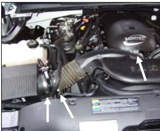
1. Disconnect the negative battery cable. Loosen the hose clamps located at the Mass Air Flow (MAF) sensor, and throttle body on the factory intake tube assembly.
