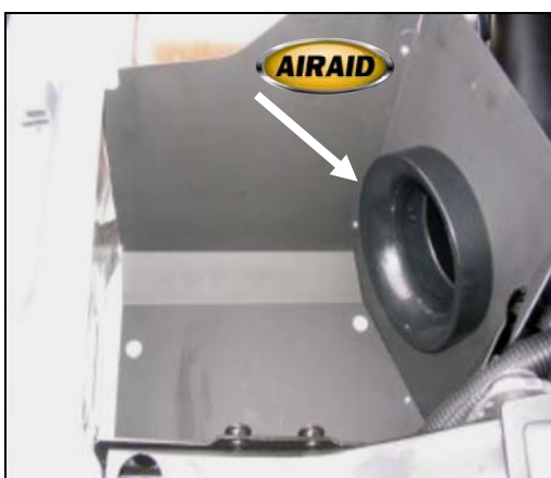
7. Install the filter adapter (#4) using three 1/4-20 x 1/2" button head bolts (#9) and 1/4" flat washers (#10). Apply the Airaid Foil Decal onto the Panel as shown.
