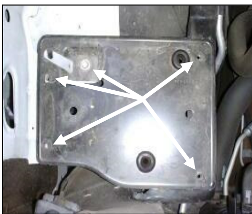
4. Using a 10mm socket, remove the five bolts that secure the factory air filter housing platform and remove it.
