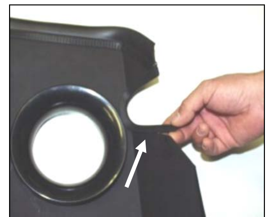
6. Install the 7 1/4" rubber trim (#12) onto the side of the Airaid Cool Air Dam.
