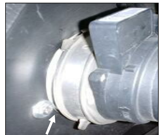
9. Slide the factory MAF meter onto the filter adapter. Tighten the hose clamp. ( Note: The factory clamp / rubber bushing must be in place on the inlet to the MAF meter. ) Reconnect the factory intake tube, MAF meter wiring harness, and tighten the clamps.
