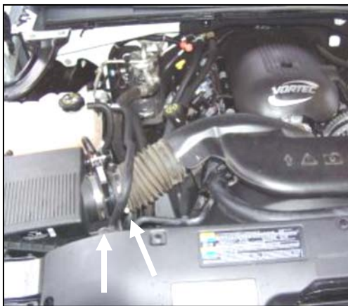
1. Disconnect the negative battery cable. Loosen the 2 hose clamps located at the Mass Air Flow (MAF) meter.
