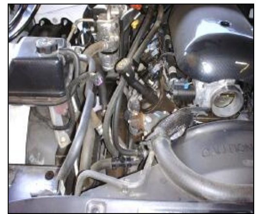
3. Remove the factory air filter lid, intake tube, and base from the vehicle as an assembly. (Hint: pull straight up on the air filter base to remove, there are no bolts, just grommets).
