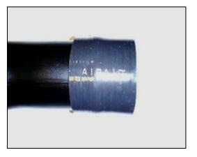
**11.** Install the urethane coupler (#7) and two #60 hose clamps (#17) onto the small end of the Airaid intake tube. (*Note: Leave hose clamps loose until final assembly.*)
