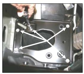
**4.** Using a 10mm socket, remove the five bolts and mounting plate from the engine compartment
