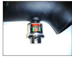
**9.** Install the factory rubber grommet and air filter minder into the Airaid intake tube.
