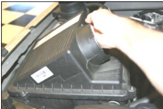
4. Grab the factory airbox and rock it back and forth, and remove it from the vehicle. It is only held in by grommets, no bolts.
