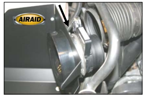
9. Re-install the Mass Air Sensor and coupler onto the air filter adapter (#4), as shown and tighten the hose clamp.
