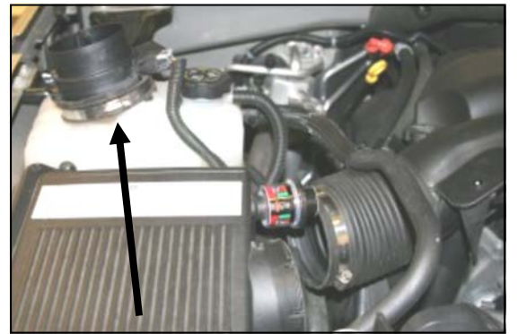
3. Without disconnecting the wiring harness, remove the Mass Air Sensor and coupler from the factory airbox, and set it aside.
