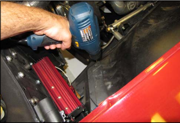
10. Drill 1/8" pilot holes into the inner fender.
