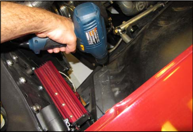
10. Drill 1/8" pilot holes into the inner fender.
