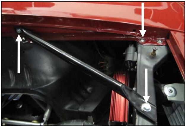
7. Remove the fender brace and the rear fender bolt on the core support. Passenger side installations require relocation of the battery and tray.
