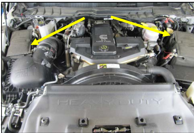
1. Disconnect The Negative Battery Terminals! Warning: Installation of this Intake system requires working in close proximity to the turbocharger. Please allow a sufficient cooling time before beginning the installation to avoid personal injury.
